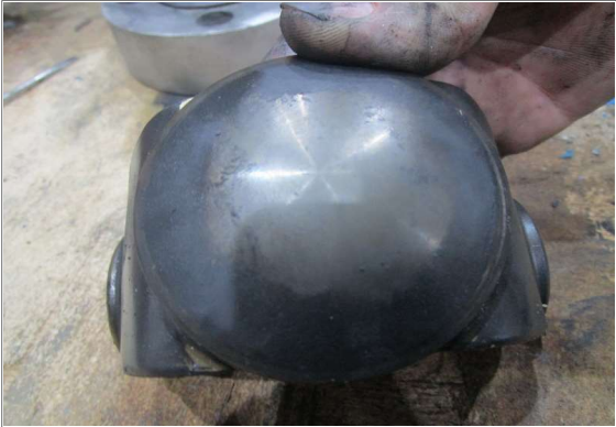
A condition of plug-seat before clean & laping.
